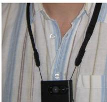
Figure 5: ViconRevue lifelogging camera (formerly Microsoft SenseCam)
