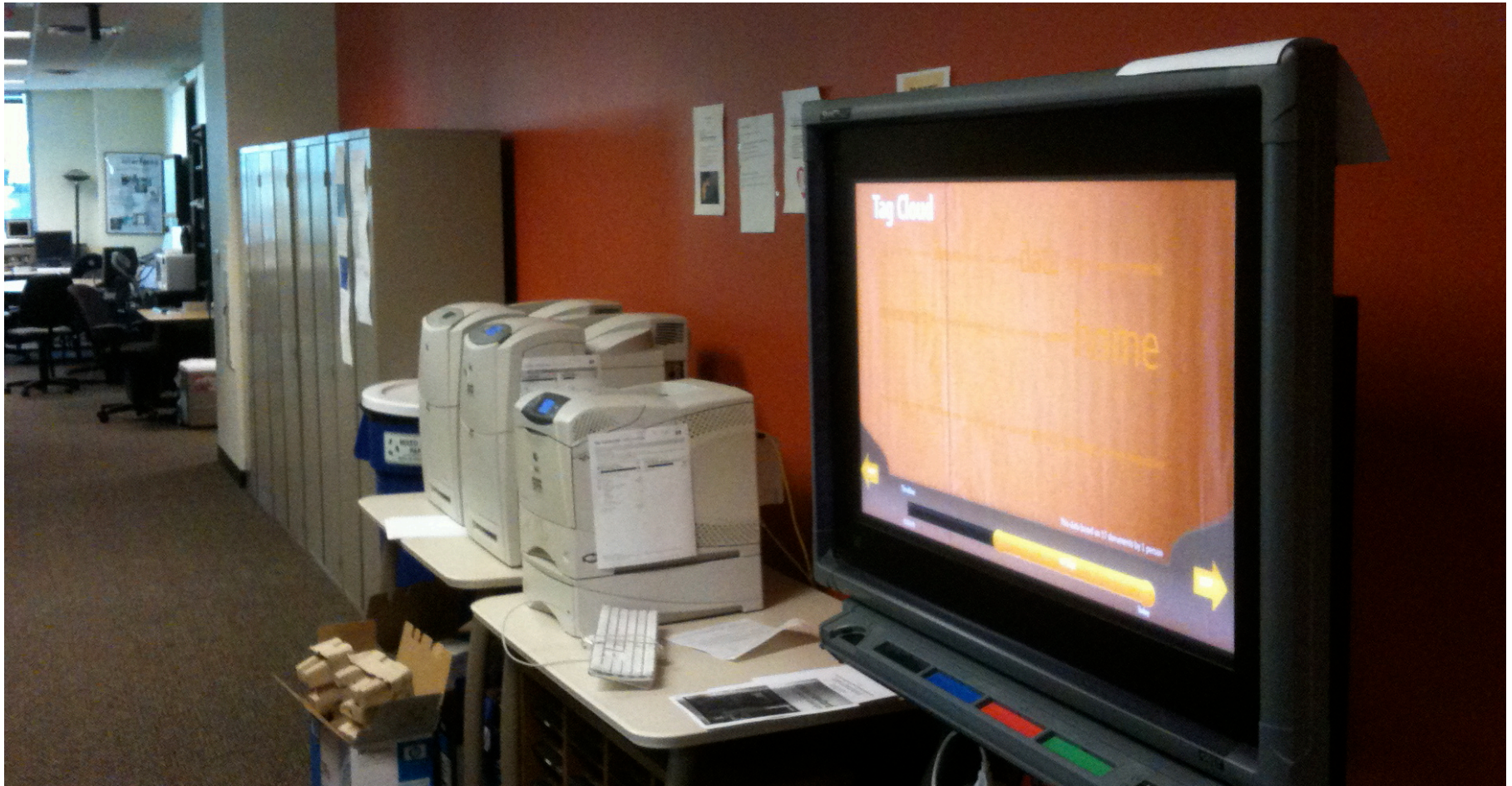
Figure 1: Imprint installed at Georgia Tech's GUV Center. Imprint runs on a 42" touch screen and cycles through a set of visualizations. Users can interact with Imprint to switch to the next or previous visualization, or scrub the dynamic query timeslider to select a timeframe from three days to three months.
